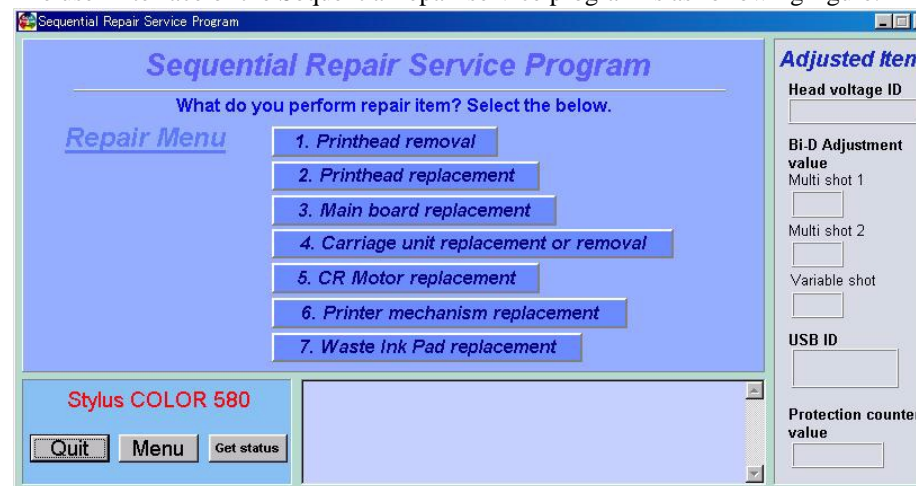
Figure 5-2. Sequential repair service program main menu
