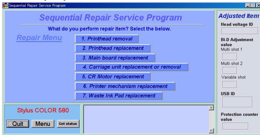
Figure 5-6. Sequential repair service program main menu
