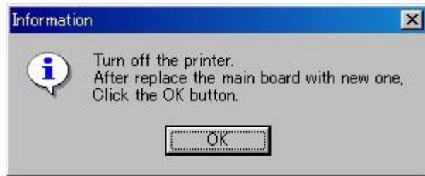
Figure 5-39. Replace the defective main board with new one.
