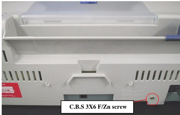
Figure 4-3. Removing 1screw for Housing
