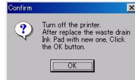
Figure 5-41. Replace the Waste drain in pad & Set the market setting
