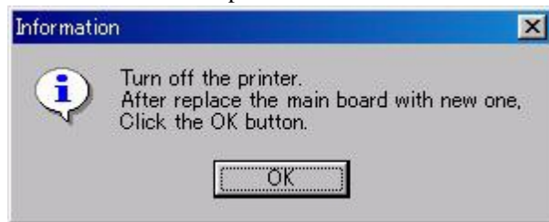
Figure 5-36. Replace the defective main board with new one
