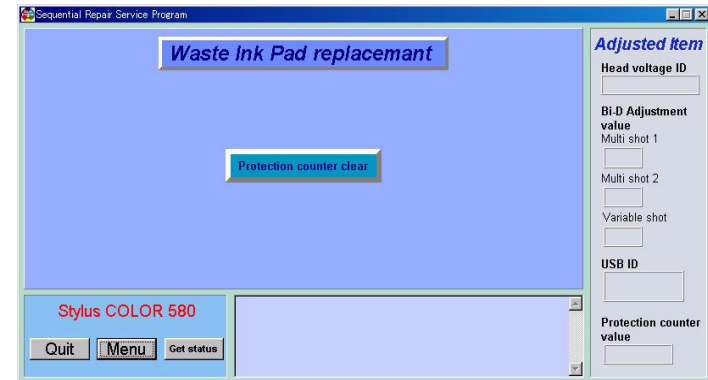
Figure 5-49. Waste drain ink pad replacement
